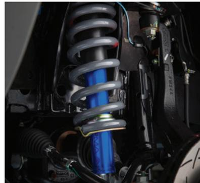
High load cargo vehicle suspension system
