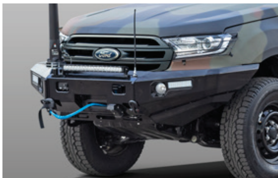
Front Bumper with electric winch and driving light
