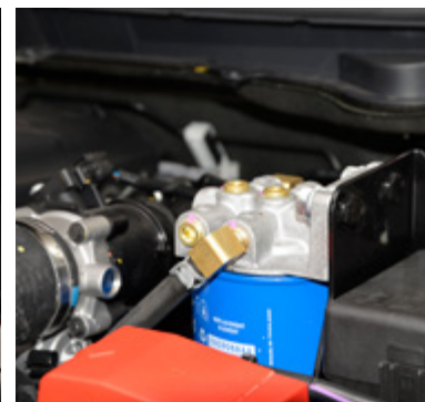
Enhanced fuel filtration system
