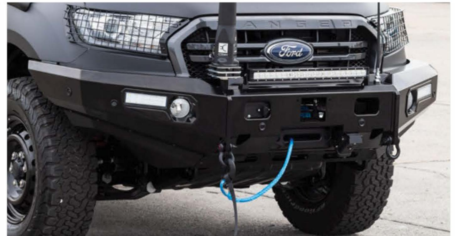
Front bumper with electric winch and LED driving light
