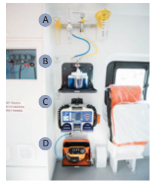
A: Oxygen therapy and vacuum kit B: Electric suction pump* C: Defibrillator* D: Portable ventilator*
